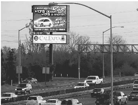
Figure 4-2. Electronic signs from Smart Sign Media use wireless technology to sense the radio stations drivers listen to, and then serve up advertisements that best fit drivers’ demographic profiles. Photo: Smart Sign Media.
